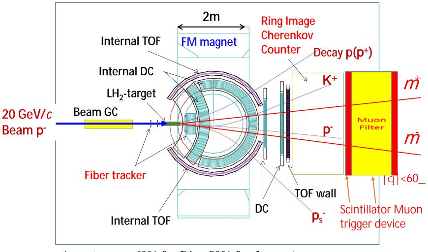
Acceptance:  $\sim 60\%$  for  $D^*$ ,  $\sim 80\%$  for decay p<sup>+</sup> Resolution:  $\mathcal{D}p/p\sim 0.2\%$  at  $\sim 5$  GeV/c (Rigidity:  $\sim 2.1$  Tm)
