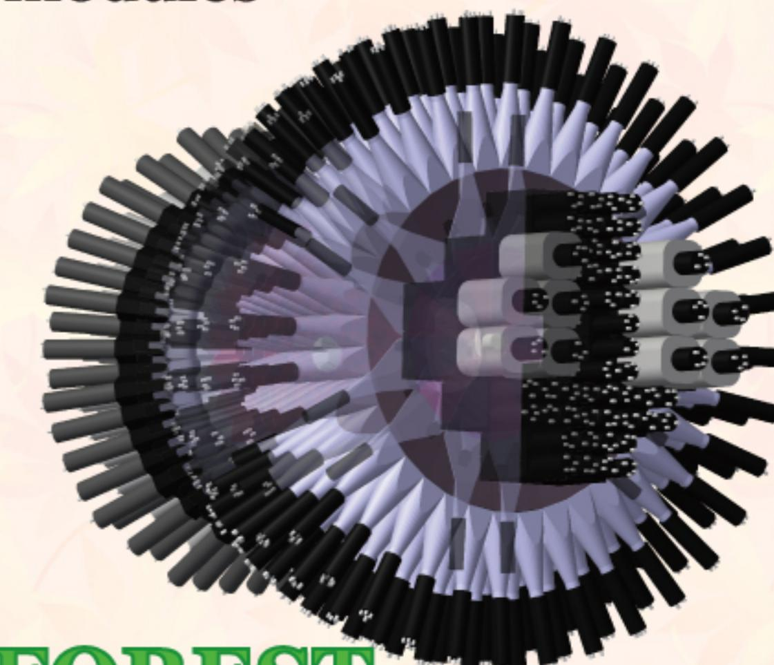
Target: 45 mm thick LH<sub>2</sub> & LD<sub>2</sub>
