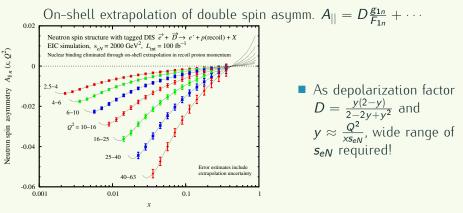
Precise measurement of neutron spin structure
